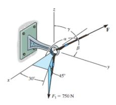
•2–73. The shaft S exerts three force components on the die D. Find the magnitude and coordinate direction angles of the resultant force. Force  $\mathbf{F}_2$  acts within the octant shown.
