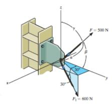
Force Vectors: By resolving  $F_1$  and F into their x, y, and z components, as shown in Figs. a and b, respectively,  $F_1$  and F can be expressed in Cartesian vector form as
