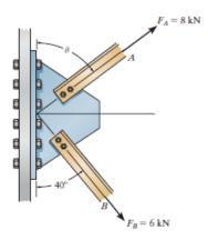
${\it Parallelogram\ Law}$ : The parallelogram law of addition is shown in Fig. (a) .
