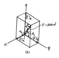
\*2–96. The tower is held in place by three cables. If the force of each cable acting on the tower is shown, determine the magnitude and coordinate direction angles  $\alpha$ ,  $\beta$ ,  $\gamma$  of the resultant force. Take x=20 m, y=15 m.
