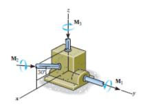
Since the couple moment is a free vector, it can act at any point without altering its effect. Thus, the couple moments  $\mathbf{M}_1$ ,  $\mathbf{M}_2$ , and  $\mathbf{M}_3$  acting on the gear deducer can be simplified, as shown in Fig. a. Expressing each couple moment in Cartesian vector form,
