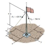
Position Vector and Force Vectors: Either position vector  $\mathbf{r}_{OA}$  or  $\mathbf{r}_{OB}$  can be used to determine the moment of  $\mathbf{F}_B$  about point O.
