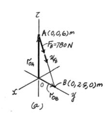
\*4-56. Determine the moment produced by force F about segment AB of the pipe assembly. Express the result as a Cartesian vector.
