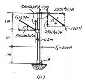
**-4–141.** Replace the three forces acting on the plate by a wrench. Specify the magnitude of the force and couple moment for the wrench and the point P(x, y) where its line of action intersects the plate.
