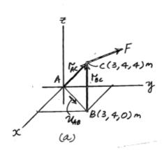
**4–58.** If  $F = 450 \, \text{N}$ , determine the magnitude of the moment produced by this force about the x axis.
