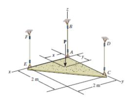
**Equations of Equilibrium:** From the free - body diagram, Fig. a,  $T_{CD}$  and  $T_{EF}$  can be obtained by writing the moment equation of equilibrium about the x and y axes, respectively.
