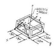
5-66. The pipe assembly supports the vertical loads shown. Determine the components of reaction at the balland-socket joint A and the tension in the supporting cables BC and BD.
