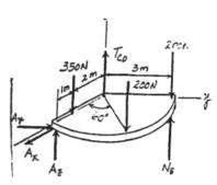
The pole is subjected to the two forces shown. Determine the components of reaction of A assuming it to be a balland-socket joint. Also, compute the tension in each of the guy wires, BC and ED.
