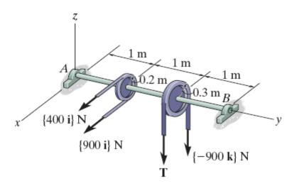
5- The shaft is supported by three smooth journal bearings at A, B, and C. Determine the components of reaction at these bearings.
