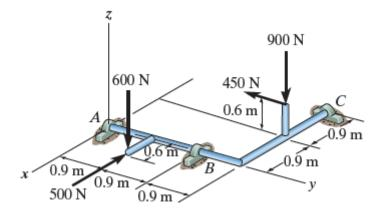
6- Determine the x and z components of reaction at the journal bearing A and the tension in cords BC and BD necessary for equilibrium of the rod.
