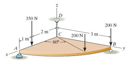
2- Determine the components of reaction acting at the smooth journal bearings A, B, and C.
