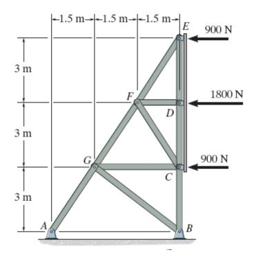
10- Determine the horizontal and vertical components of force that the pins at A,B, and C exert on their connecting members.
