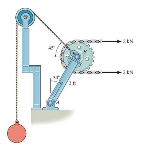
14- Determine the reactions on the collar at *A* and the pin at *C*. The collar fits over a smooth rod, and rod *AB* is fixed connected to the collar.
