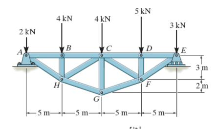
8- Determine the force in members *JE* and *GF* of the truss and state if these members are in tension or compression. Also, indicate all zero-force members.
