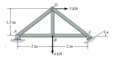
2- Determine the force in each member of the truss, and state if the members are in tension or compression.
