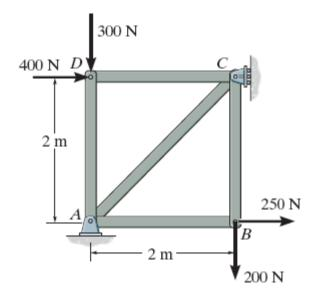
3- Determine the force in each member of the truss, and state if the members are in tension or compression.
