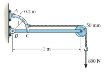
11- Determine the greatest force P that can be applied to the frame if the largest force resultant acting at A can have a magnitude of 2 kN.
