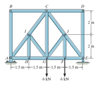
9- Determine the force in members *FG*, *GC* and *CB* of the truss used to support the sign, and state if the members are in tension or compression.
