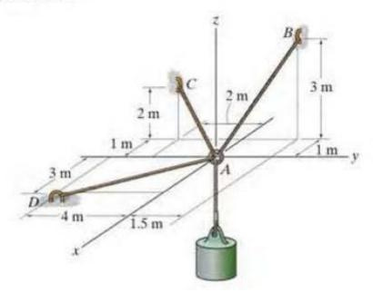
**3–74.** The lamp has a mass of 15 kg and is supported by a pole AO and cables AB and AC. If the force in the pole acts along its axis, determine the forces in AO, AB, and AC for equilibrium.
