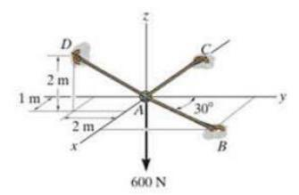
**3–47.** The shear leg derrick is used to haul the 200-kg net of fish onto the dock. Determine the compressive force along each of the legs *AB* and *CB* and the tension in the winch cable *DB*. Assume the force in each leg acts along its axis.
