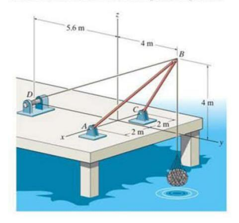
**3–55.** If the mass of the flowerpot is 50 kg, determine the tension developed in each wire for equilibrium. Set x = 2 m and z = 1.5 m.
