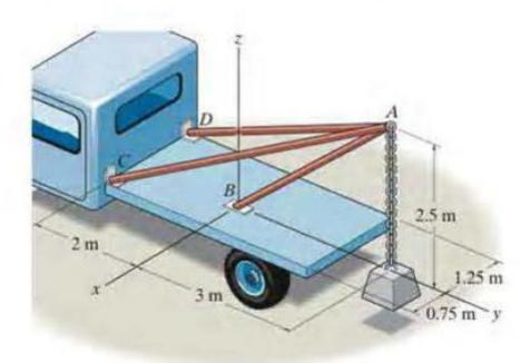
•3–57. The ends of the three cables are attached to a ring at A and to the edge of the uniform plate. Determine the largest mass the plate can have if each cable can support a maximum tension of 15 kN.
