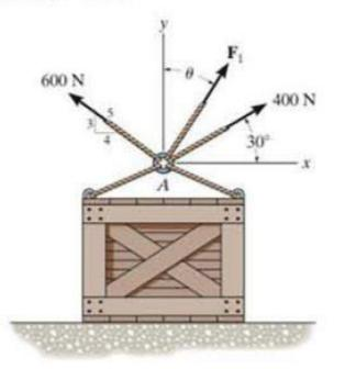
**2–46.** The three concurrent forces acting on the screw eye produce a resultant force  $\mathbf{F}_R = 0$ . If  $F_2 = \frac{2}{3} F_1$  and  $\mathbf{F}_1$  is to be 90° from  $\mathbf{F}_2$  as shown, determine the required magnitude of  $\mathbf{F}_3$  expressed in terms of  $F_1$  and the angle  $\theta$ .
