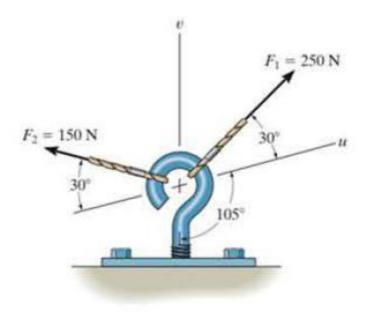
\*2-24. If the resultant force  $\mathbf{F}_R$  is directed along a line measured 75° clockwise from the positive x axis and the magnitude of  $\mathbf{F}_2$  is to be a minimum, determine the magnitudes of  $\mathbf{F}_R$  and  $\mathbf{F}_2$  and the angle  $\theta \leq 90^\circ$ .
