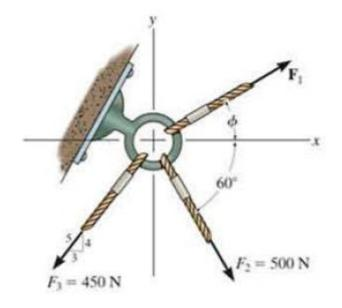
\*2-40. Determine the magnitude and direction measured counterclockwise from the positive x axis of the resultant force of the three forces acting on the ring A. Take  $F_1 = 500$  N and  $\theta = 20^\circ$ .
